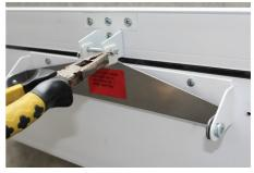
Remove the two pivot screws from the lower part of the transit plate and retain for future use.
