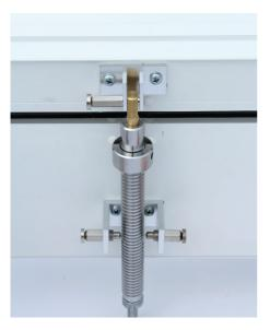
Wind the chrome nut down the chrome threaded section until it engages with the two quick release pins on the lower bracket. Ensure some downward force is applied to the opening frame so that the seals make firm contact.
